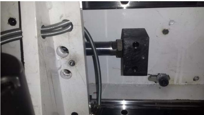
5) Spin the block off to extend the stroke length
